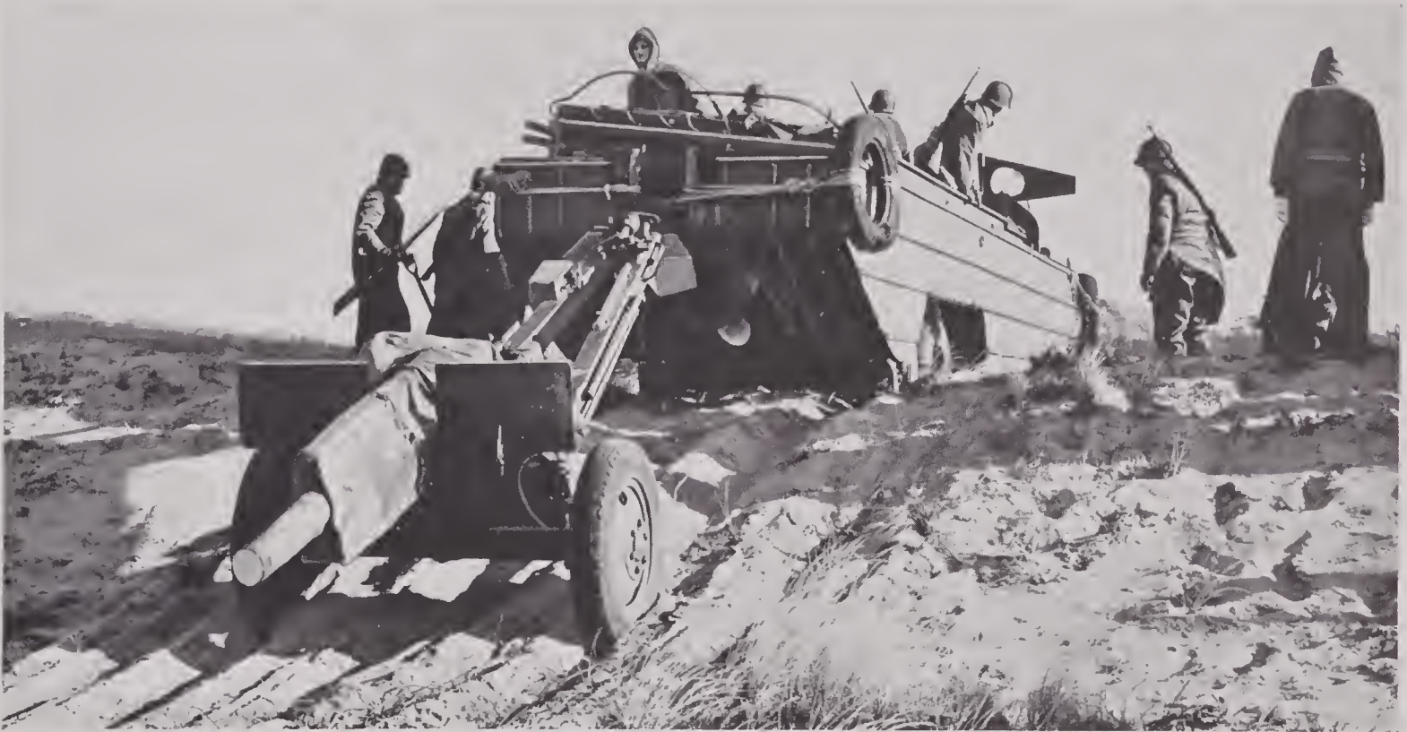
FIGURE 95. DUKW takes role of prime mover to haul howitzer over Provincetown sand dunes.
